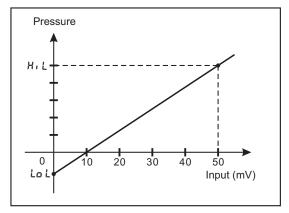
(1). When using the "Resistance Transmission Pressure Gauge" as the pressure sensor, the input signal parameter 5n must be set to PrE, set  $H_L$  to the full scale value of the sensor, set LoL to 0.
